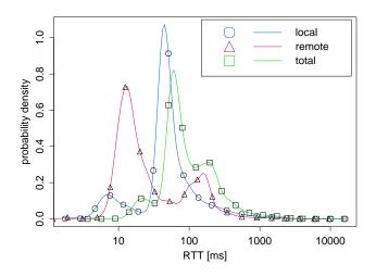
Figure 10: TCP round trip times for trace SEP.
