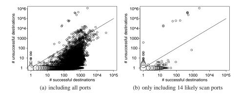
**Fig. 1.** Scatter plot showing number of successful vs. unsuccessful connections with remote IPs per DSL line, computed for a single day of the ISP trace. The size of the circles is proportional to the number of lines having the corresponding ratio.
